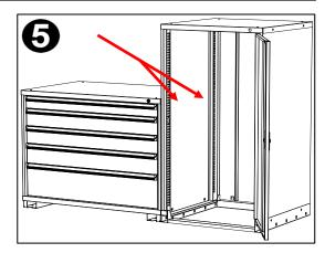
Close door to ensure proper function and adjust as needed. Finish tightening fasteners with tools. Remove installation bracket and dispose of properly. Ensure swing door has free motion. Shim and/or adjust level as needed.
