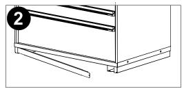
Push base cap closed and slide into the other forklift channel.
