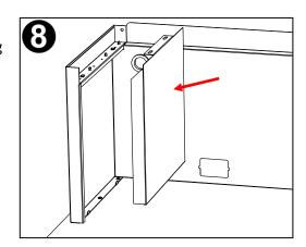
Install beams by engaging the lance in beam support with notch in beam. Slide beam until spring pin locks in place.
