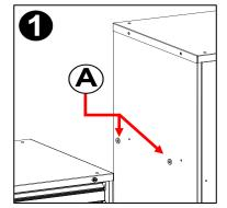
Position garage into place. Ensure garage is level to adjacent units.
