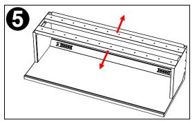
Verify that holes on underside of riser beams are facing toward inside.
