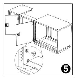
Close door to ensure proper function and adjust as needed. Finish tightening fasteners with tools.
