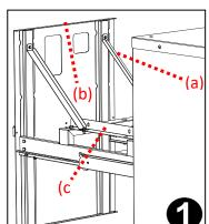
Remove drawer body from housing by releasing safety clips on slide profile and then lifting drawer while pulling out.
