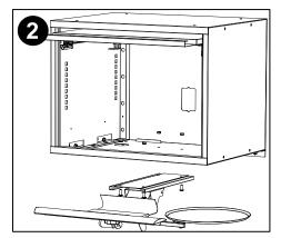
Replace retained bottom pan and adjust keyboard mount as desired.
