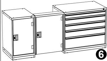
Remove installation bracket. Check for free motion of swing door. Shim and/or adjust level as needed. Properly dispose of bracket and hardware.
