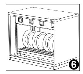
Route hose/cord from each reel through corresponding roller guides and attach proper stopper ring.
