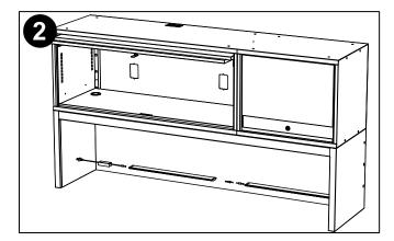
Place light, hook-up power supply, and interconnect wires for adder units. Clean up wiring as desired.
