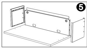
Align sides over marked hole locations and attach with supplied MDC-0723 screw qty. 6. Refer to photo below.
