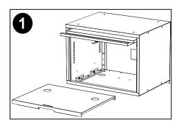
Use supplied MDC-0006 washer qty. 4 and 10167-01 nut qty. 4 to attach keyboard mount. Insert bolts through keyboard mounting plate and tighten Keps nuts from inside cabinet (4 places).
