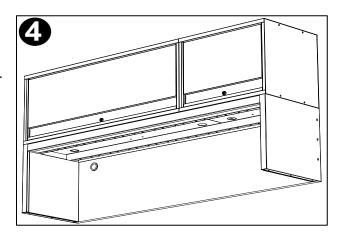
Use supplied MDC-0006 washer qty. 4 and 10167-01 nut qty. 4 to attach keyboard mount to underside if riser by placing bolt through keyboard mount first and tightening Keps nut in riser cabinet.
