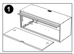
If mounting to riser kit (A), proceed to step (4). If wall mounting, anchor wall cleat in desired location (B).
