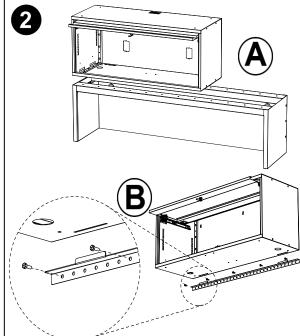
To finish installation of wall mounted upper cabinet, integrate cabinet with wall cleat and anchor cabinet back to wall. Proceed to step (5) for information regarding mounting adjacent cabinets and finishing installation.
