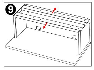
Verify holes on underside of riser beams are facing toward inside.
