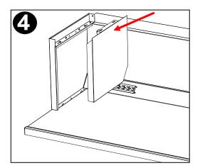
Install beams by engaging lance in beam support with notch in beam. Slide beam until spring pin locks in place.
