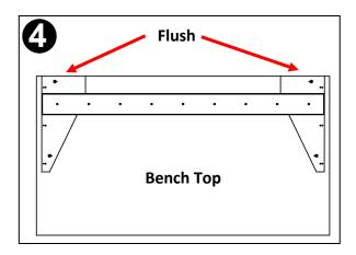
Set riser back panel on back edge of bench top and attach side panels by engaging three (3) lances in the sides with three (3) slots on back panel.
