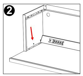
Using supplied MDC-0723 screw qty. 1 refer to photo above, drill into bench top through hole on back side of back panel.
