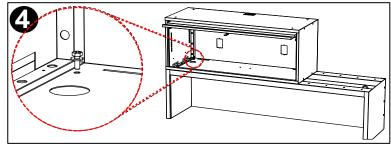
If mounting adjacent cabinets, work from one side mounting cabinets to either wall cleat or riser kit, linking cabinets with supplied 94383-53 screw qty. 4 and 94394-71 nut qty. 4 at all four (4) locations on side of cabinet.
