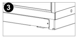
Kick plate notches should integrate with forklift channels and snap into place.
