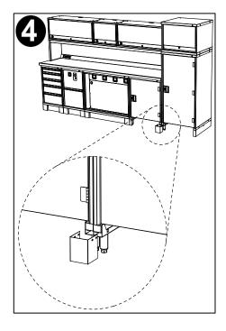
Once all kick plates are in place, adjustments may now be made. Obrounds allow kick plates to move forward and back ensuring a flush appearance at front of unit. Obrounds on swing doors allow for vertical adjustments. After desired look is achieved, check all screws to ensure all kick plates are securely fastened. To access stainless steel leveling feet, remove screws from kick plate.
