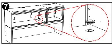
Close doors ensure proper function of lock.
