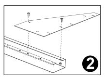
(Optional) Connect additional hardware through holes with circle indicators to help stabilize template assembly.
