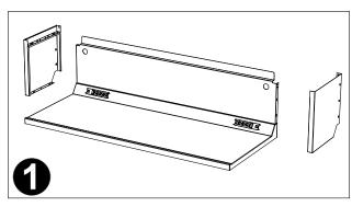
Move assembly side to side on bench top to desired location and mark hole locations. Align sides over marks and attach with supplied MDC-0723 screw qty. 6. Refer to photo.
